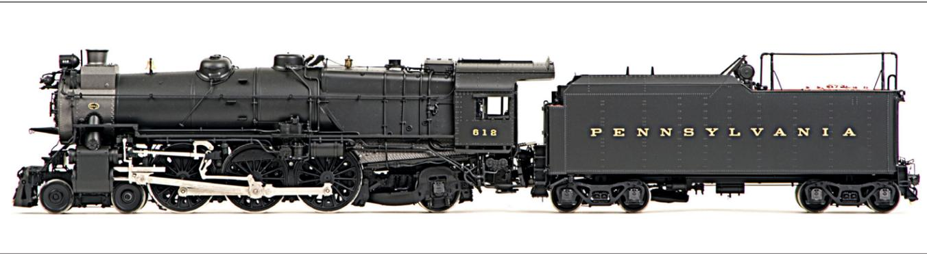
**(above & cover)** 'K-4sa' #612 with a special radio antenna equipped 130P75 tender. The most distinguishing feature of the 'sa' is the front-end throttle box mounted on the top of the smokebox. The 'sa' also had larger driving cylinders and a variety of other unique details, although the basic configuration is the same as the 'Post-War' version described on the previous pages. The K-4sa modified locomotives were the 'hot rods' of the class. (post 1952 service period)
